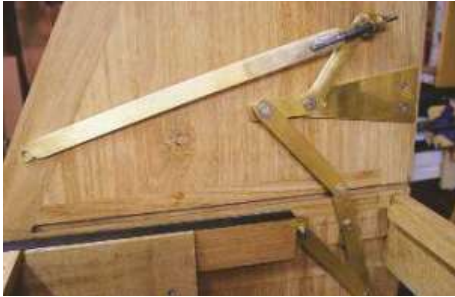
▲ Pic 12 The loper mechanism in its closed position. There are several pivoting and fixed points for the brass components
